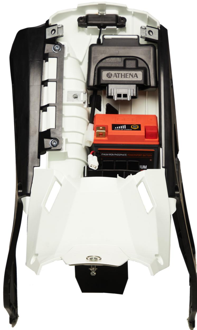
To develop this new model, the Vertigo R&D engineers have been working hand by hand with GET. The outcome is a revolutionary battery-assisted electronic injection system, which in all respects improves and facilitates the start of the bike while optimizing the operation of its electrical components.
